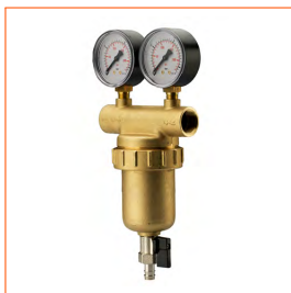
FI 00. Self-cleaning filter with 2 manometers, removable cartridge and discharge tap.
