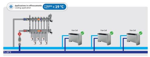
In this first application example, AQUASTOP XL is used to interrupt the cold water supply to an entire collector. It is important to note that in this case the device should be installed immediately downstream of the branch and as close to it as possible.
