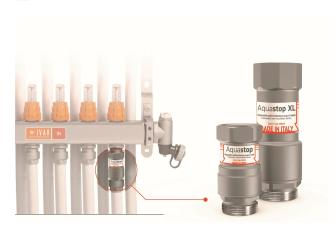
AQUASTOP - AQUASTOP XL are cold water circulation of cold water that can be applied upstream of heating elements upstream such as radiators or towel warmers in order to prevent, in the case of a mixed heating and air conditioning heating and air conditioning systems, cold water from circulating in them, which can cause problems in summer, such as dripping condensation.
