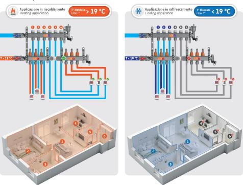
In this second application example, AQUASTOP XL is used to section off a manifold, with circuits 1 to 3 always supplied and circuits 4 to 6 supplied for heating only. This is a cost-effective solution compared to installing three different AQUASTOPs on circuits 4, 5 and 6.
