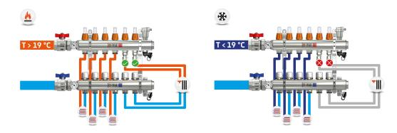
AQUASTOP can be installed upstream of heating elements such as radiators or towel warmers to prevent water from circulating inside them and causing problems such as dripping condensation in summer.
