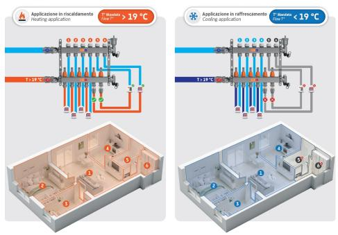
During winter operation, circuits 5 and 6 on which AQUASTOP is installed are regularly supplied with hot water. In summer operation, on the other hand, AQUASTOP interrupts the supply of cold water both on circuit 5, dedicated to the radiator, and on circuit 6, intended for the radiant floor. This prevents the formation of condensation on the radiators or in particularly humid environments such as the bathroom.
